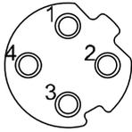
**BUS IN: M12 4-pin socket, D-coded**
