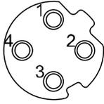
**BUS OUT: M12 4-pin socket, D-coded**
