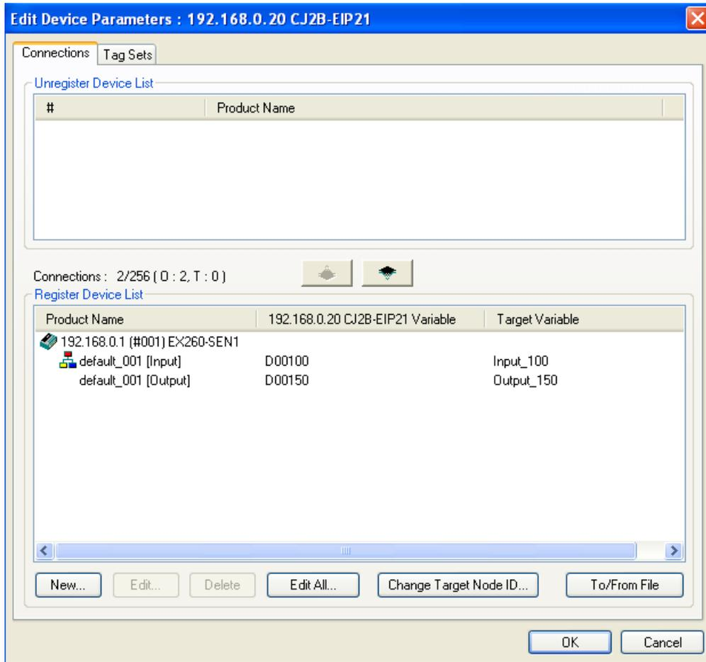
Example: Tag Set D00100 (2 bytes) to the Input, and D00150 (4 bytes) to the Output.
