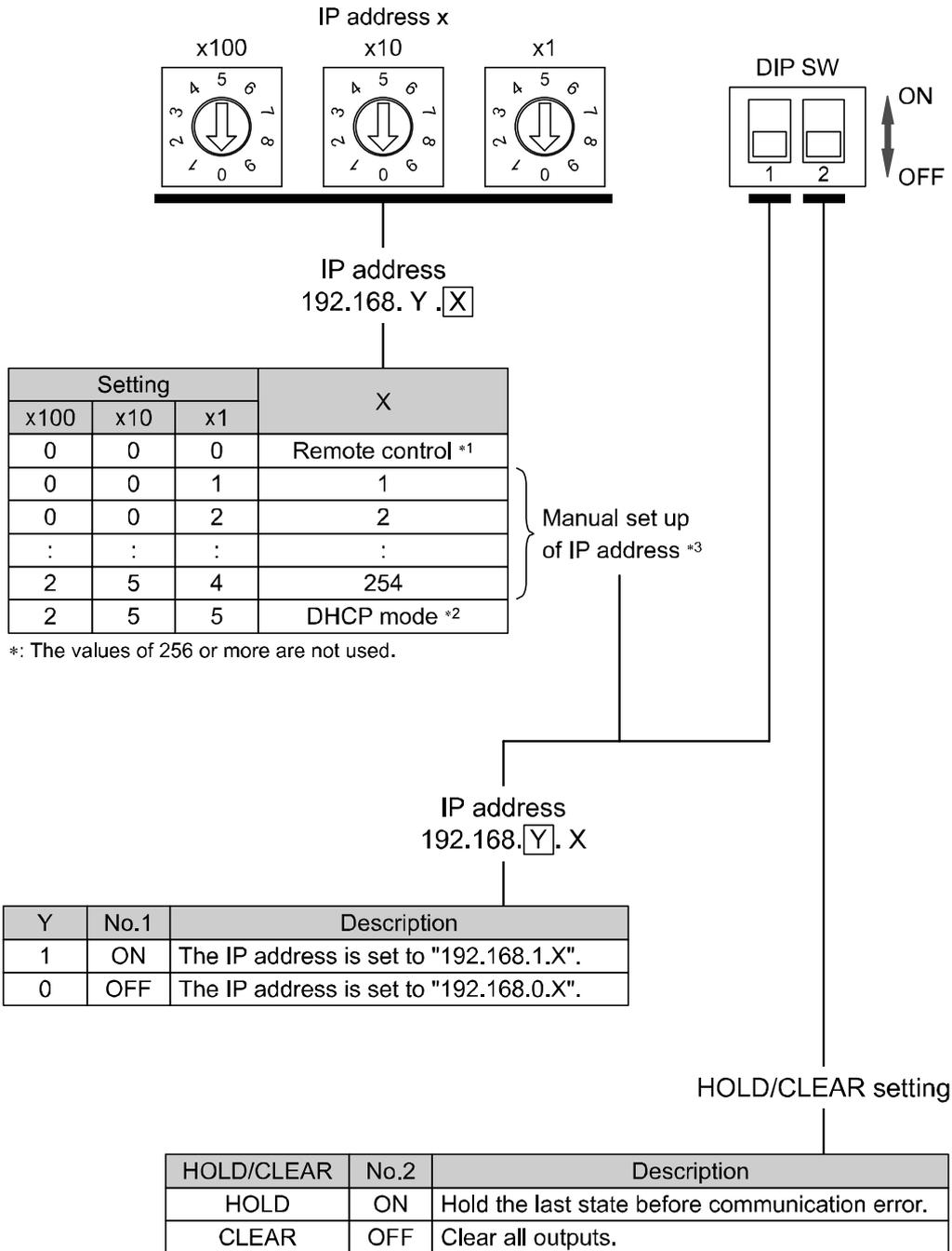
\*1: Remote control (IP Address X switch set to 000)
