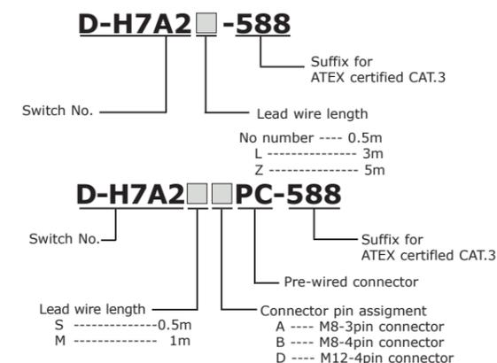
This product is a Solid State Auto Switch of direct mounting specification of the installation PNP output type.
