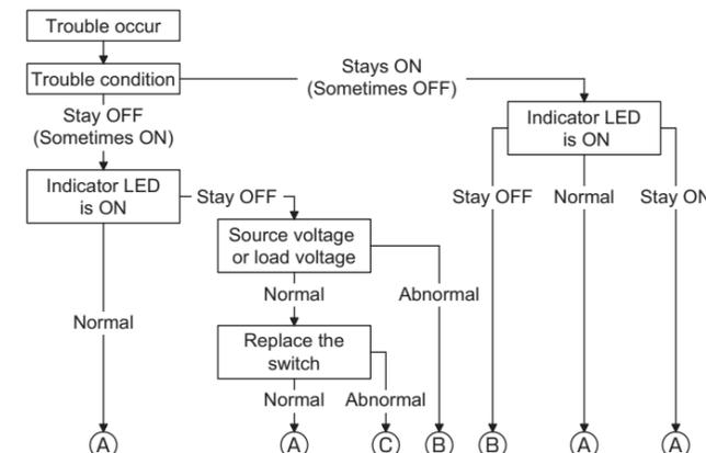
A --- Switch output parts failure(replace)
