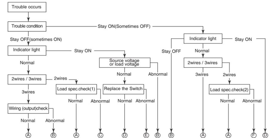
Load spec. check(1) ----- ON voltage > Load voltage-Internal voltage drop
