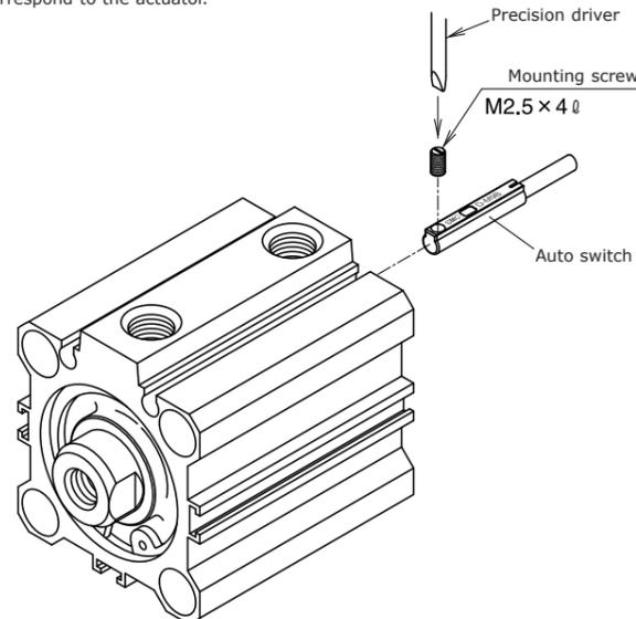
M2.5 mount screw tightening torque shall be 0.1 to 0.2Nm.
