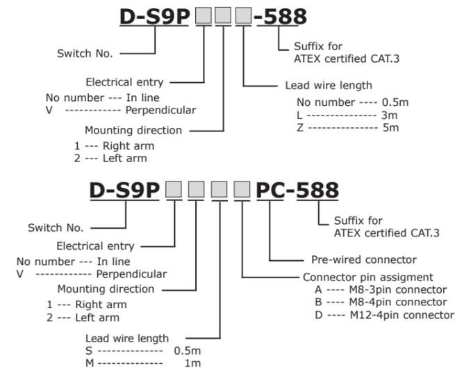
This product is a Solid State Auto Switch of direct mounting specification of the installation PNP output type.
