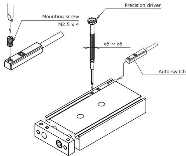
M2.5 mount screw tightening torque shall be 0.05 to 0.1Nm
