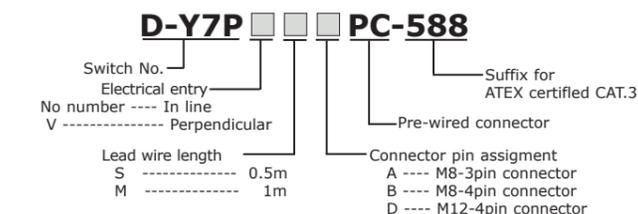
This product is a Solid State Auto Switch of direct mounting specification of the installation PNP output type.
