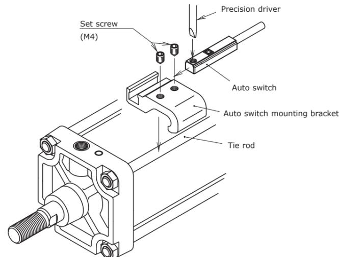
M4 set screw tightening torque shall be 1.0 to 1.2Nm
