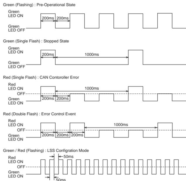
LED Indication of SI unit is based on CANopen Specification (CANopen Spec.DR-303-3). Refer to DR-303-3 Indicator Specification for details.
