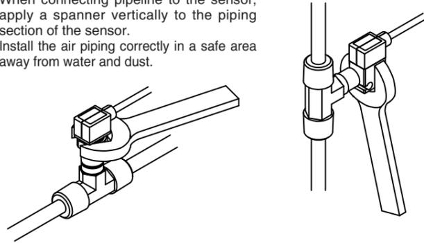
Hold the sensor and insert it into the one-touch fitting carefully and securely all the way to the bottom.
