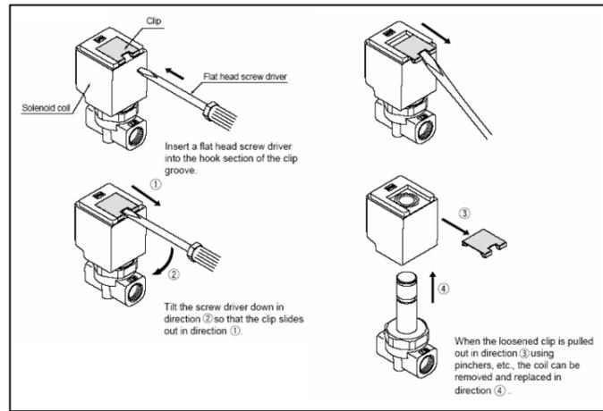
After replacing the coil, the clip is reinstalled by pushing it back in the direction opposite to its removal.
