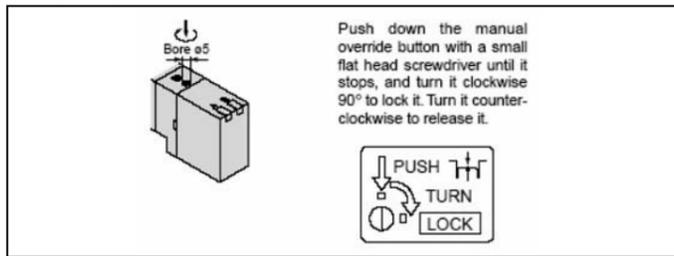
Push down the manual override button with a small flat head screwdriver until it stops, and turn it clockwise 90° to lock it. Turn it counterclockwise to release it.
