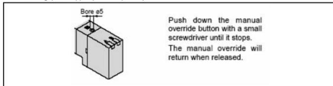
Push down the manual override button with a small screwdriver until it stops. The manual override will return when released.
